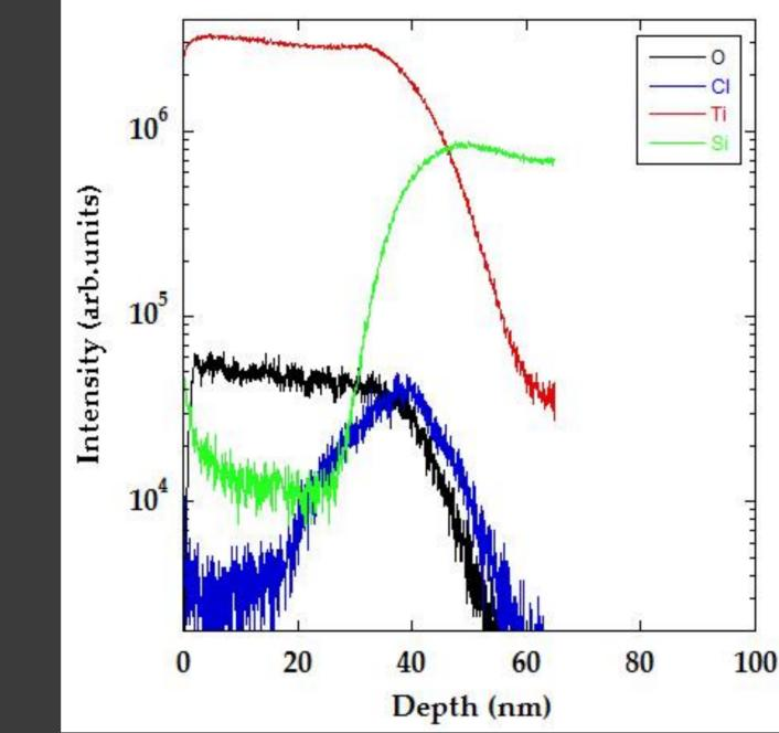
TiO<sub>2</sub> films grown on 40 °C and 250 °C using plasmaenhanced ALD. Spectra recorded were by measuring positive ions of Ti and Si (using 3 keV  $O_2^+$  primary ions), and negative ions of O and Cl (with 5 keV Cs<sup>+</sup> primary ion beam).
