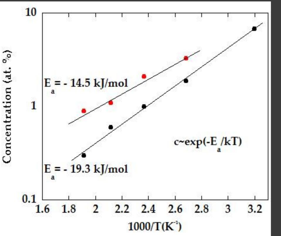
Arrhenius plot of CI concentration vs reciprocal temperature (1000/T) for samples grown by thermal ALD and PEALD. The linear fitted lines were used to calculate the activation energy.
